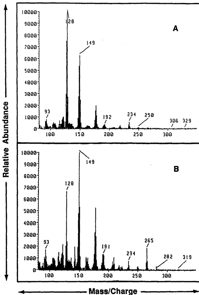
Figure 10. Mass spectra of 1'-deoxy- $^2\text{H}$ -ABA methyl ester eluted at a retention time of 9.26 min (A) and peak at a retention time of 9.59 min (B) shown in the purified 1'-deoxy- $^2\text{H}$ -ABA samples
