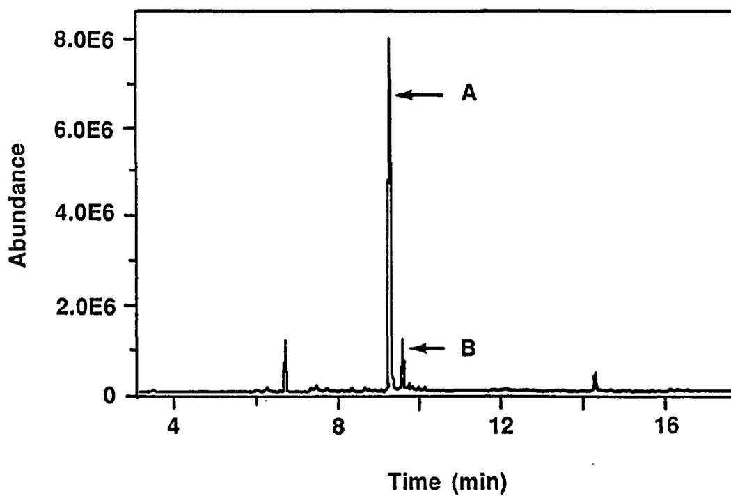
Figure 9. Total ion chromatogram of the methyl ester of purified 1'-deoxy-<sup>2</sup>H-ABA
