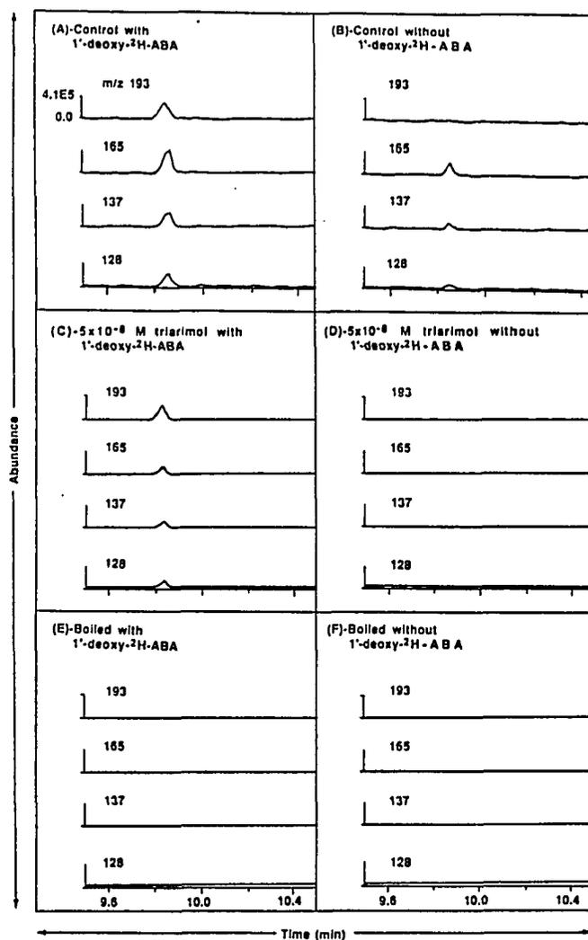
Figure 11. Ion chromatograms of  $m/z$  193, 165, 137, and 128 obtained by GC-MS of extracts from cultures grown and resuspended in the absence (A, B) or presence (C, D) of  $5.0 \times 10^{-8}$  M triarimol, and boiled cultures without triarimol (E, F). Profiles A, C, and E represent cultures fed with 1'-deoxy- $^2$ H-ABA, while B, D, and F are from cultures without feeding
